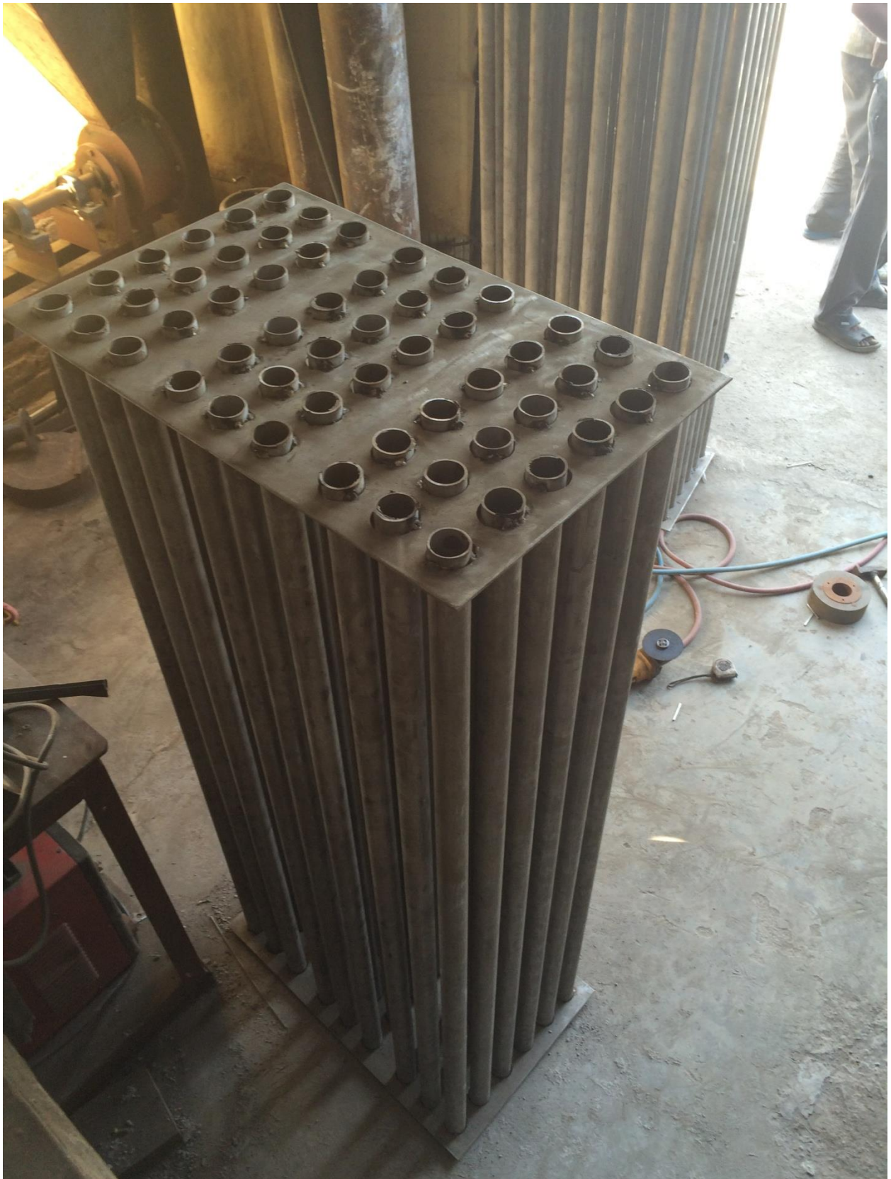
Figure 12: A view of the heat exchanger during manufacturing process
