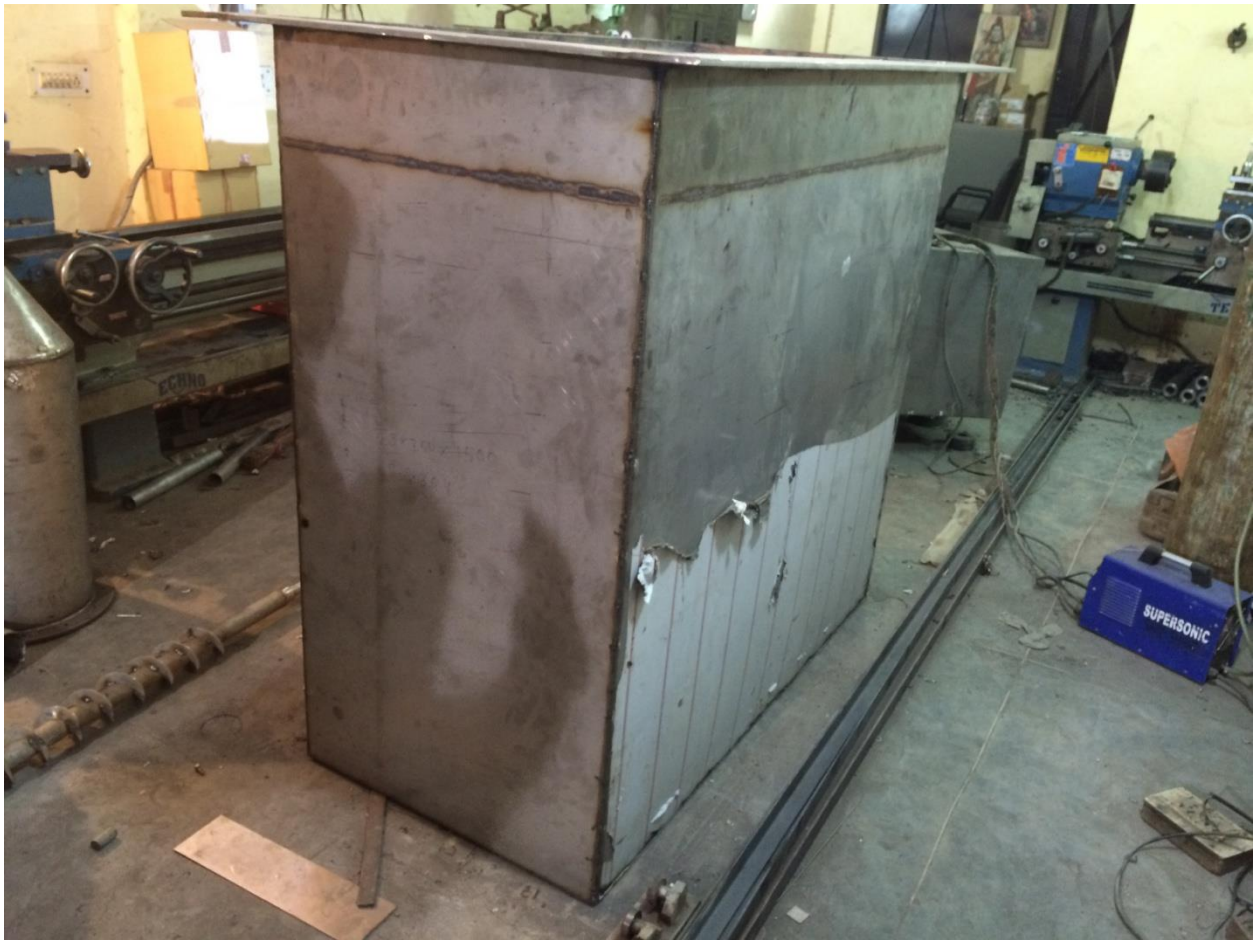
Figure 13: A view of the Hotgas filter
