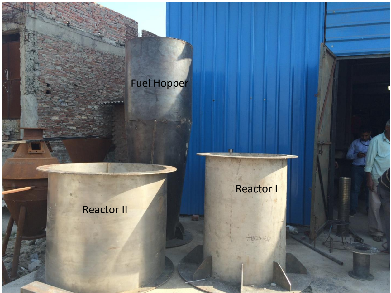
Figure 11: A view of the fuel hopper with the gasification reactors during the manufacturing process
